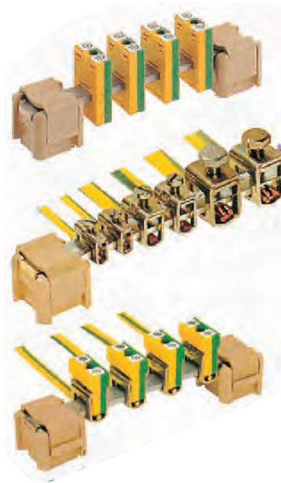
In order to bring together neutral conductors and protective conductors at a central point, it is advantageous to use ZB tension clamps together with 10 x 3 or 6 x 6 busbars. The tension clamps can be pushed onto the busbar and adjusted to the entire wiring in the system.
