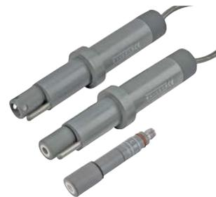
The optional differential preamplifier or 4 to 20 mA transmitter, and temperature compensation element are in the housing, and are not thrown away when the electrode needs replacement. The electrode is powered by the controller it is connected to, so the signal is always preamplified and there are no batteries to go dead.
