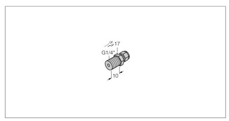
Compression fittings for direct mounting of TP temperature probes
