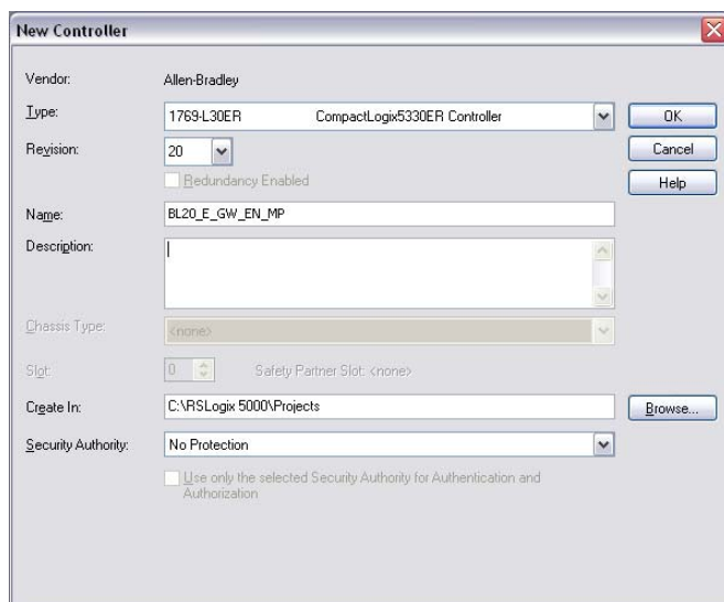
Figure 5-1: Configuration of the controller
