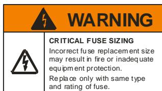
P/N 49455 – Replace Fuse only with one of same type and range. Incorrect fuse size may result in equipment damage.
