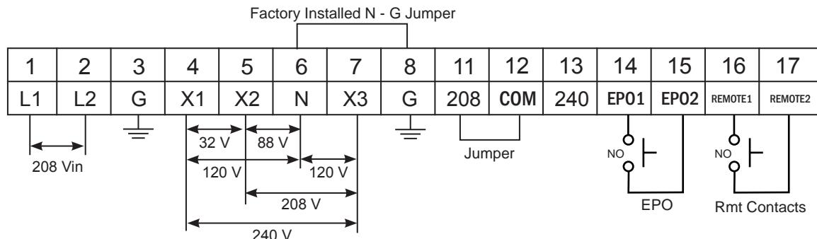
**240 Vin** – Using provided jumper, connect terminals 13 – 12.
