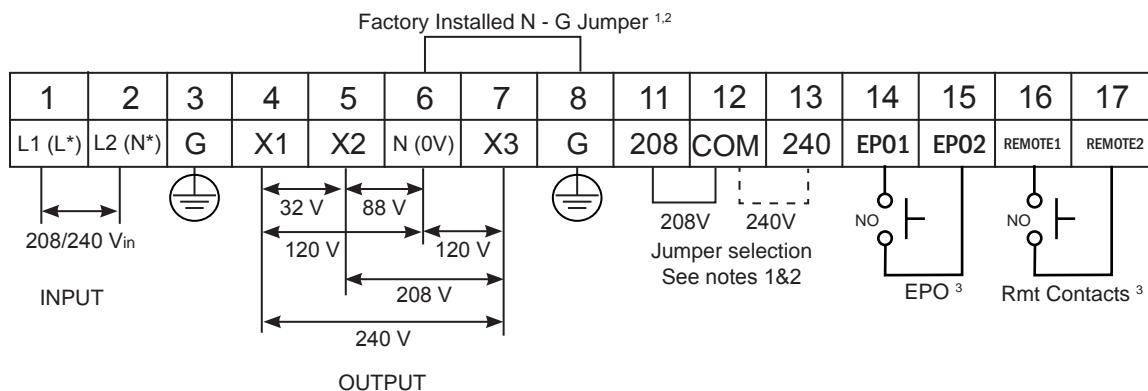
\* – If only one input line is hot, connect hot line to terminal 1 (L), and connect the Neutral line to terminal 2 (N).
