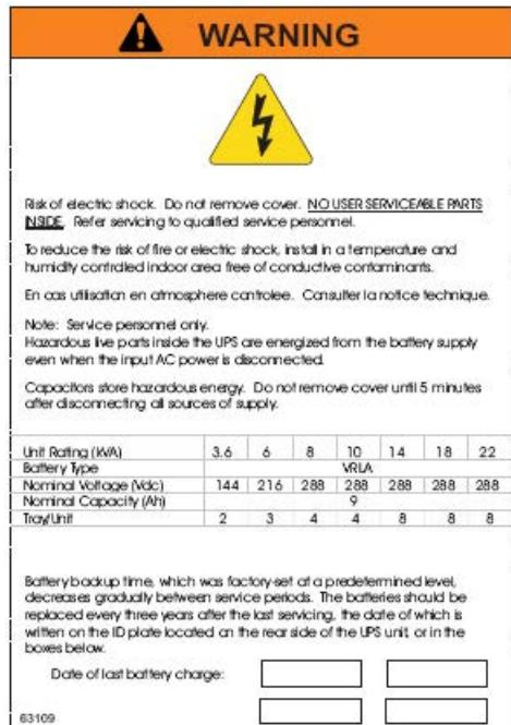
P/N 63109 – There are no user-serviceable parts behind cover. Wait five minutes after disconnecting the UPS to allow the internal capacitors to discharge completely.
