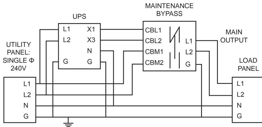
See the application instructions included with the External Maintenance Bypass Unit for wiring details.
