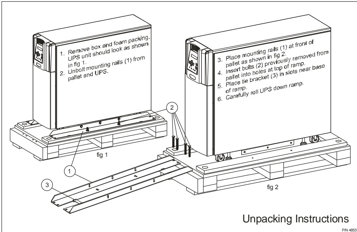
4. Retain the shipping rails for use as permanent mounting of the UPS.
