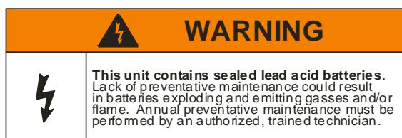
P/N 49455 – UPS Batteries require annual preventative maintenance. Failure to perform regular maintenance could result in batteries exploding, or emitting gasses or flame.
