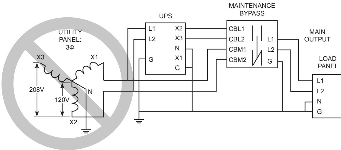
**DO NOT USE 3-PHASE INPUT WHEN USING AN EXTERNAL MAINTENANCE BYPASS**
