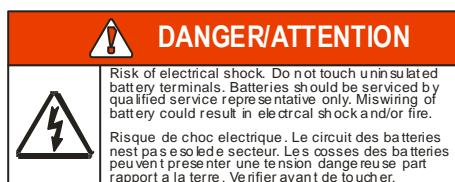
P/N 48518 – Battery terminals can deliver dangerous electrical shock. Service by qualified service representatives only.
