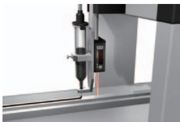
Controlling the height of a dispenser nozzle
