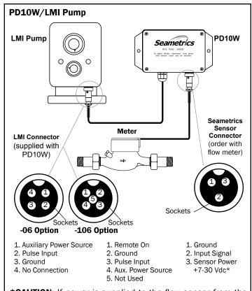
**\*CAUTION:** If power is supplied to the flow sensor from the PD10, ensure that the voltage supplied to the sensor does not exceed the sensor's allowable maximum input voltage.
