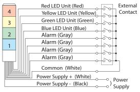
\*KJ-110/112/120 are voltage-contact type, therefore have no alarm signal wires. \*Only the KJB has Gray wires for alarm input.
