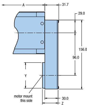
Parallel motor mounting is employed whenever a shorter overall unit length is needed. The motor is positioned along the sides or bottom of the table as designated by position A, B, or C. (No coupling required)
