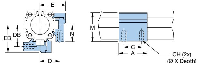
Type D1 (with two internal threads)
