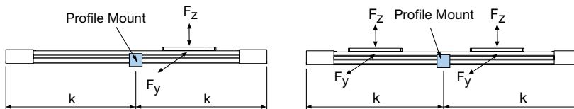
The greater the load and/or the longer the unsupported length between mounts, the more the actuator is susceptible to deflection.
