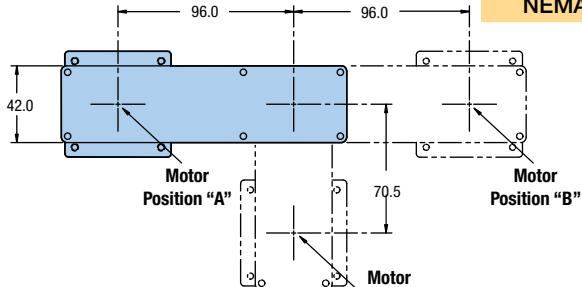
Note: Some sensor pack and encoder restriction apply when mounting motors larger than NEMA 23 in the A or B positions. Please consult factory.
