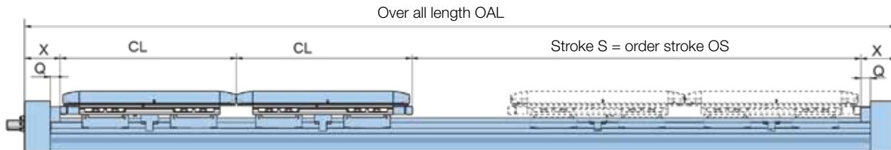
Order stroke OS = Effective stroke ES + 2 x Safety stroke SS + Carrier distance CD (not shown)
