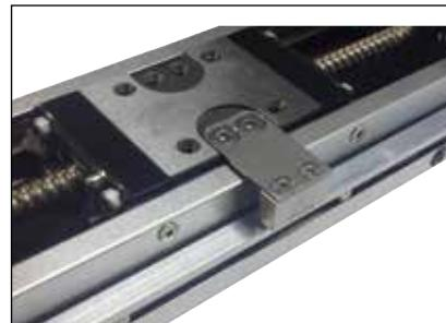
Limit sensor mounting screws are reverse-thread style so tightening the screw loosens the limit sensor in the track and vice versa.
