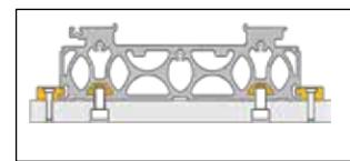
Pinning options are also available for mounting, carriage to base and carriage to carriage. Consult factory for additional information.
