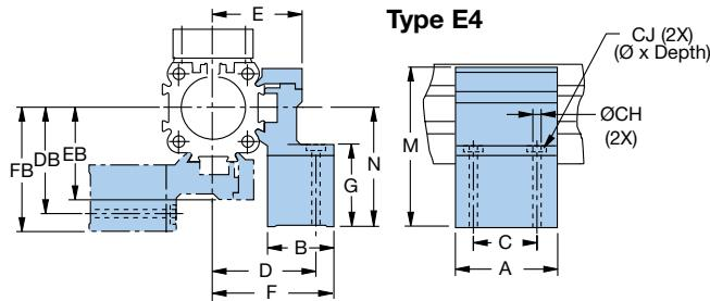
Type E1, E2, E3 and E4 (with two thru holes)
