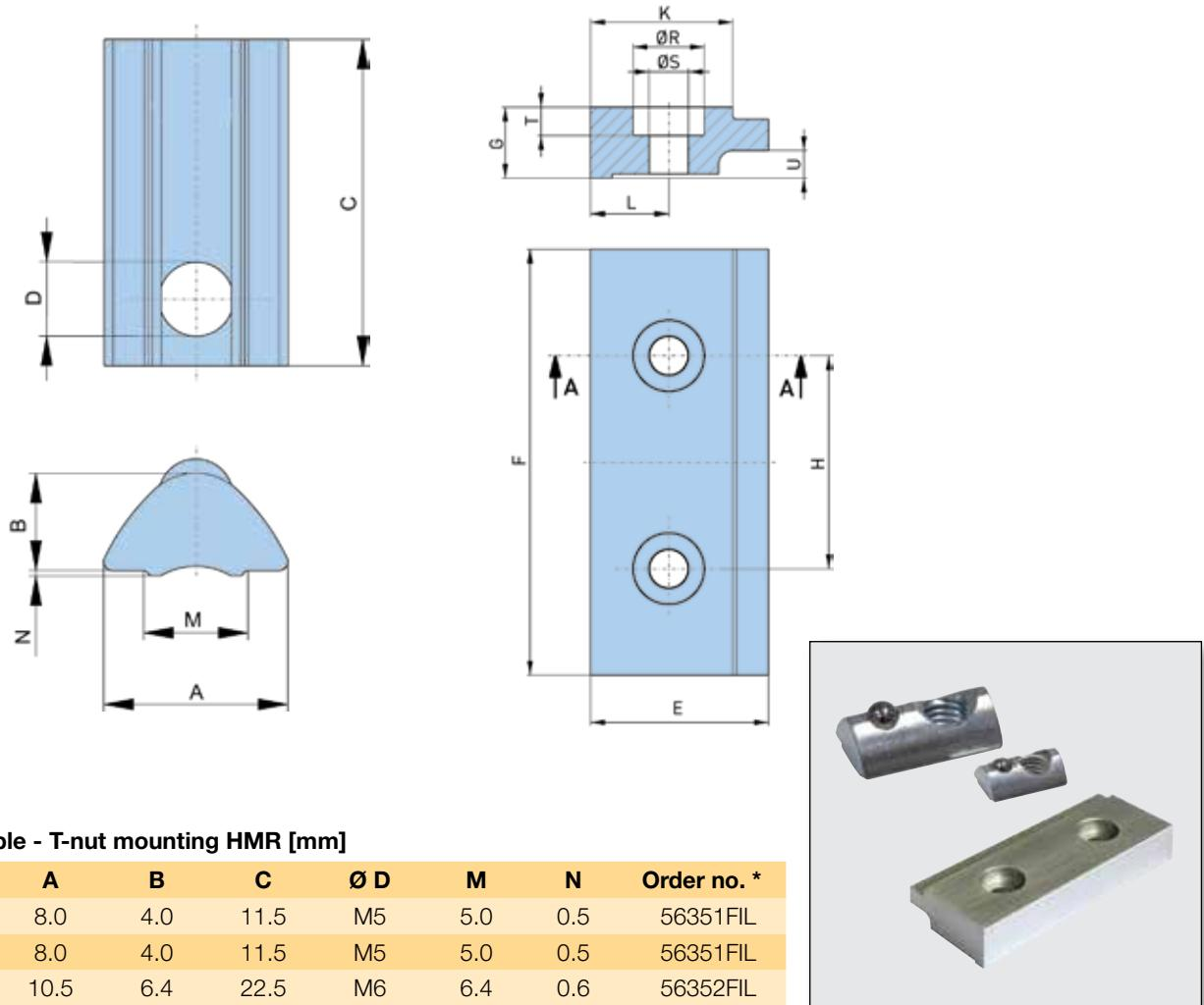
**Dimension table - T-nut mounting HMR [mm]**
