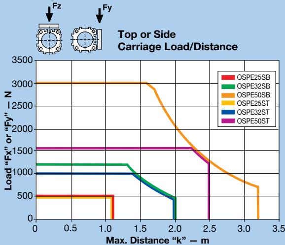
**Maximum Permissible Unsupported Length****Determining end cap and profile mounting placement**
