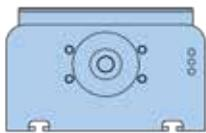
**Reinforced profile** - for long un-supported spans (i.e. gantry style applications).
