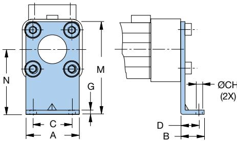
**Type B1 and B4 – Reinforced End Cap**
