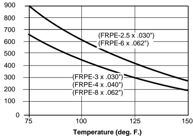
Suggested working pressure of polyethylene is 1/3 of burst pressure at system operating temperature.
