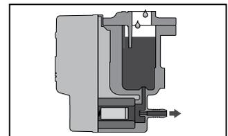
3. The condensate is discharged from the outlet port, due to the system pressure acting on the top of the liquid.
