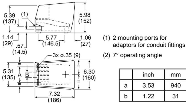
**Notes:** These Foot Pedal Operators come assembled with switch PXBB1921 (Normally Passing). With the pedal in the unoperated position, the switch is in the actuated non-passing position. With the pedal actuated, the switch is in the unactuated Normally Passing position.
