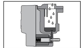
Level monitoring and discharge operation are continuous.
