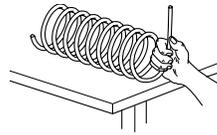
Position bulk length coils on work table extending away from you, cut-end up in 12:00 o'clock position.
