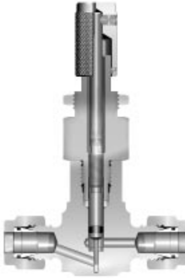
Figure 1: NS Series Metering Valve with Knurled Knob Cross Sectional View
