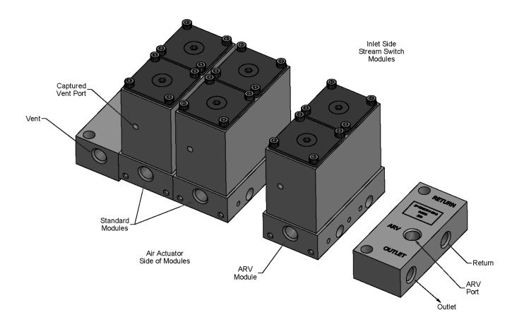
The improved features on the Stream Switching Units are included on the ARV Modules. This includes the Captured Vent and Enhanced Position Indicator. It is provided with a new end block which has a dedicated atmosphere reference port. Also, the re-designed ARV Modules can be used with Fast Loop Filtration.
