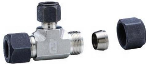
As a lubricant or anti-galling device it is twice as effective as the common internally silver plated nut used in other fittings of this type. For example, the average make-up torque for a CPI™ tube fitting (“moly” coated nut) is roughly half that of a silver plated nut. This is because the moly is a lubricant while the silver plate only provides a differential metal bearing surface which still requires lubricant.
