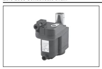
Zero air loss condensate drains are designed for economical removal of unwanted water, oil emulsions, and other liquids. These drains will only open when liquid is present and will not allow any compressed air to escape from the system.
