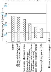
The bars in the graph indicate the sensing range (typical) for the respective material. However, there is a slight variation in the sensing range depending on the product. Further, if there is a
