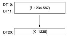
Converts real number data (range: +32767.49 to -32768.49) specified by S to signed 16-bit integer data (rounding the first decimal point off to integer) when the trigger turns on. The converted data is stored in D.
