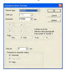
Select "Transfer" from "File" in the menu bar. The "transfer data" screen will open. Select "Condition" to open "Communication Setting" screen. Change the value for "Timeout".Click "OK" button to complete the change of setting.
