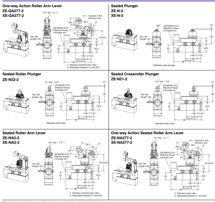
Note: 1. Unless otherwise specified, a tolerance of ±0.4 mm applies to all dimensions. 2. The diagrams shown the Switches with two, M4 screws (length: 45) attached. (The screws are provided.)
