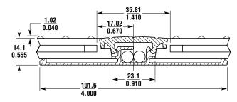
2-Part Joining Trim: PN 43222-0096 Joining Trim Aluminum Base: PN 32592 Joining Trim Cover Black: PN 32591 Joining Trim Cover Yellow: PN 32591-0010
