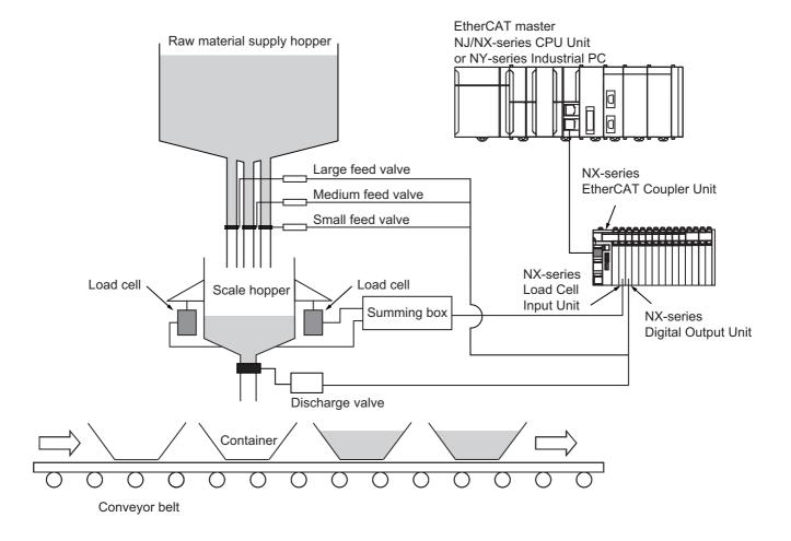
With discharge weighing, the raw material that was loaded into the scale hopper beforehand is discharged into a container and once the net weight of the discharged raw material reaches the fixed weight, discharging stops. As the raw material is discharged from the scale hopper, the net weight of the raw material in the scale hopper decreases.
