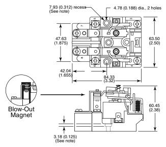
Note: Recess for screw mounting on units with 300-600 VAC coils
