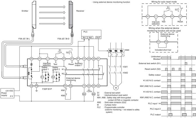
\* Auxiliary output 1 gives inverted signal of safety output (default setting).
