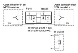
Note: 1. Residual voltage in the output section of Proximity Sensors or Photoelectric Sensors becomes less than 0.5 V because the current flowing from terminals 1 or 3 is as small as approx. 10 μA, allowing easy
