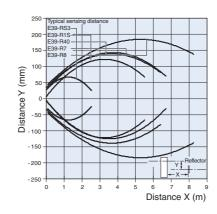
Retro-reflective Models (radial) E3F2-R2R□41-□ (polarizing) and reflectors
