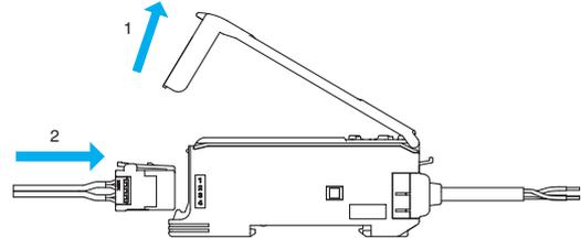
To remove the connector, press down on the locking lever and pull the connector out.
