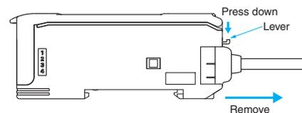
**Mounting and Removing Amplifier Units**
