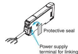
**Note:** Attach the seals to the sides with grooves.
