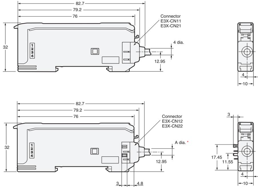
Amplifier Unit with Connector for Sensor Communications Unit
