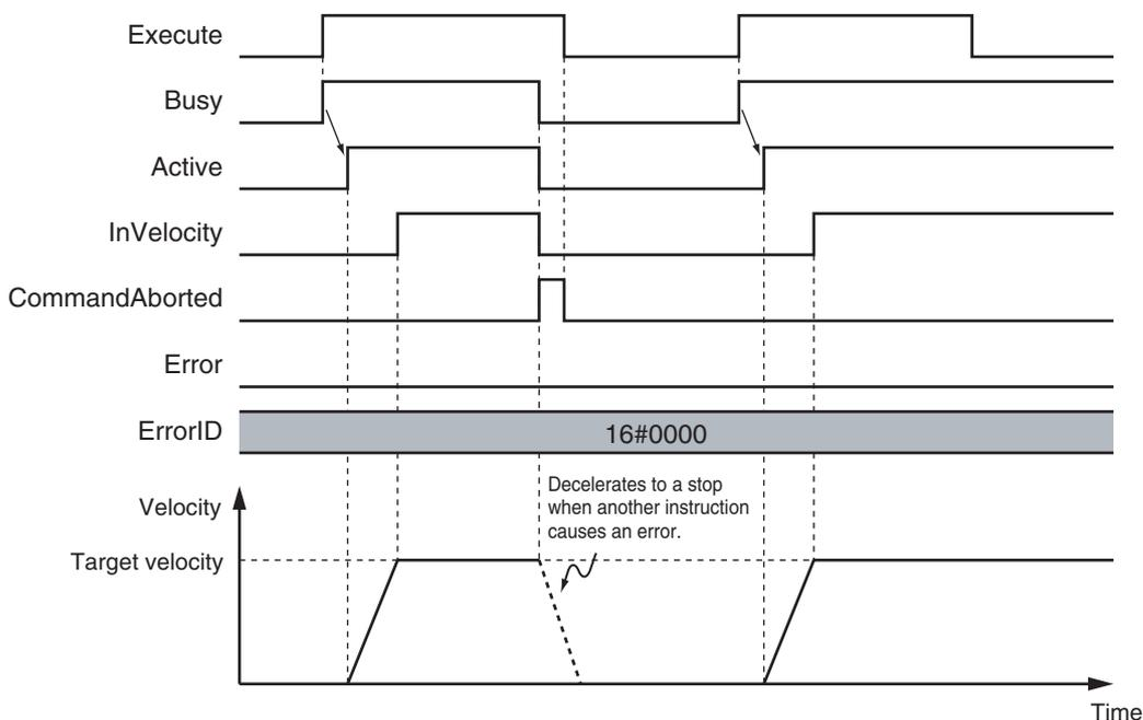
The MC Function Module uses Position Control Mode of the Servo Drive or other device and sends target position commands to achieve the specified target velocity.
