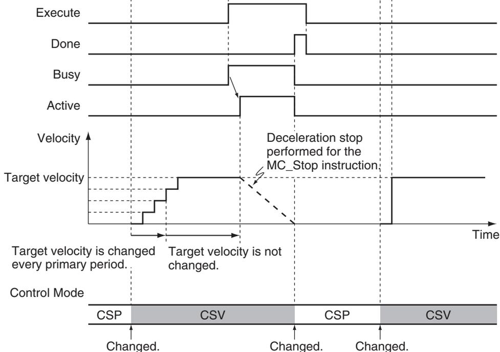
The Servo Drive will receive commands in the velocity control loop. Therefore, if any disturbance causes the velocity to decrease below the command velocity, no change in velocity will occur to remove the following error.
