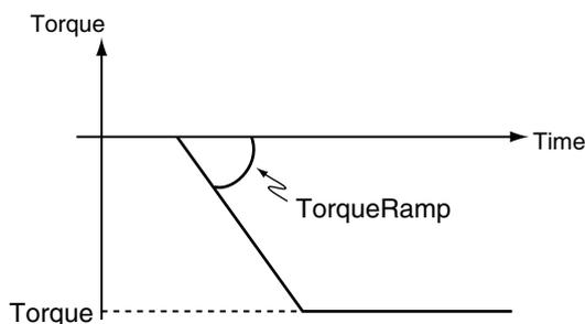
The MC Function Module uses the Torque Control Mode of the Servo Drive. The Servo Drive receives the torque command value from the MC Function Module in the torque control loop and to control the torque. You can specify the velocity limit value for the Servo Drive in the *Velocity* (Velocity Limit) input variable to the motion control instruction. You can use this to limit high-speed revolution of the motor when the load on the motor is low in Torque Control Mode.
