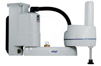
The Omron Adept Cobra<sup>™</sup> s800 Inverted robot is an affordable, highperformance overhead mounting SCARA robot system for mechanical assembly, material handling, packaging, machine tending, and screw driving. It is ideal for mounting above a conveyor belt, increasing the footprint efficiency. Adept Cobra s-Series robots include the Adept SmartController<sup>™</sup> motion controller, which provides performance capabilities unmatched in the industry.
