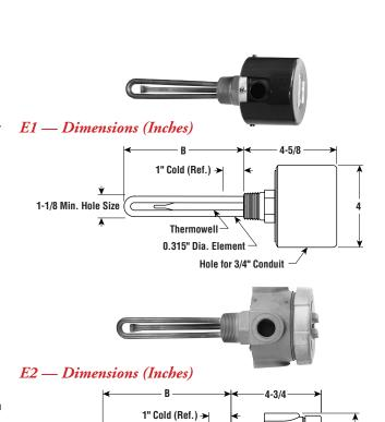
Thermowell 0.315" Dia. Element 3/4" NPT Conduit Opening -
