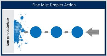
The Minncare Dry Fog 2 System produces and ultrafine droplet size that tends to bounce off of hard surfaces and thus avoid excessive condensation, corrosion and surface wetting issues associated with a fine mist bio-decontamination procedure.
