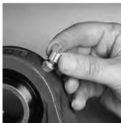
2. Place a Zerk-Lock onto the fitting
