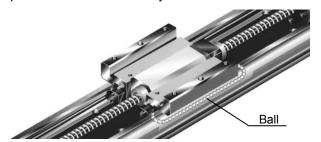
There is no longer metal noise generated by colliding balls and thus noise is reduced. Since balls are aligned by retainers, annoying noise decreases. Wear caused by friction between balls decreases, oil no longer runs out due to contact, and lubricating oil collects at the retainers. Accordingly, operation becomes smooth.
