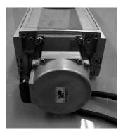
$/\!\!\!\! \cap$  Caution: The cable exit direction must be the same for the motor to be removed and replacement motor to be installed.
