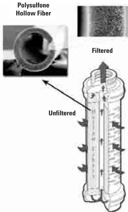
The FiberFlo HF Cartridge line has been tested to produce a sterile effluent when challenged with bacteria according to Health Industry Manufacturer's Association (HIMA) standards.
