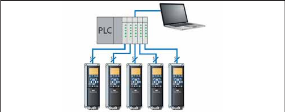
Fig. 8.7 Traditional wiring. No fieldbus
