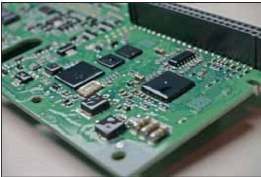
Fig. 9.8 Printed circuit board with conformal coated
