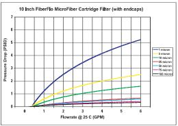
Cartridges are challenged at 3 to 5 GPM/10" on a single pass with a water based slurry of either SAE-Fine or SAE-Coarse test dust depending on the micron rating. The efficiencies are derived by measuring the ratio of upstream versus downstream particle counts taken on an automated particle counter.
