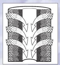
The true gradient density of these filters results in particle entrapment throughout the depth of the media, reducing surface blinding and providing increased filter life and dirt holding capacity.
