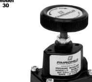
The Model 30 is designed for applications that require high capacity and accurate process control in a small package. A poppet valve which is balanced by utilizing a convoluted diaphragm, insures a constant output pressure even during wide supply pressure variations. Stability of regulated pressure is maintained under varying flow conditions through the use of an aspirator tube which adjusts the air supply in accordance with the flow velocity.
