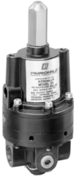
The Model 25 Reversing Relay provides an output which will decrease in direct proportion to an increase in input pressure.
