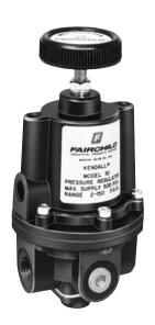
The Model 10 is designed for applications that require high capacity and accurate process control. A poppet valve which is balanced by utilizing a rolling diaphragm, insures a constant output pressure even during wide supply pressure variations. Stability of regulated pressure is maintained under varying flow conditions through the use of an aspirator tube which adjusts the air supply in accordance with the flow velocity.
