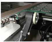
For linear applications, the Tru-Trac™ can be mounted above or below the moving object, and the tension on the wheel can be adjusted for a wide range of applications, such as packaging, conveyors, mail sorting, cut-to-length, labeling, gantries, etc.
