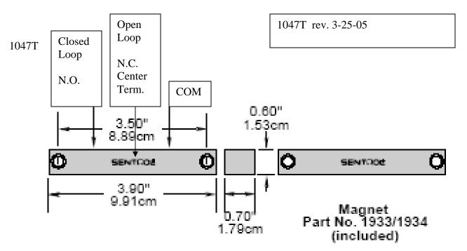
N.C. Normally Closed Contact Terminal Marked Open (Open Loop)
