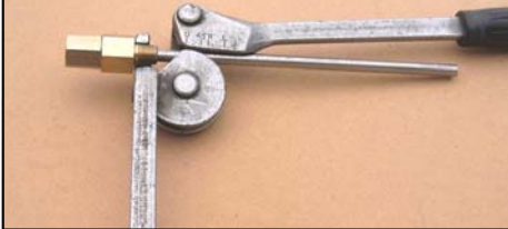
Bend the Pitot Tube & Disassemble
