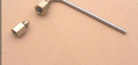
Bend the Pitot Tube & Disassemble
