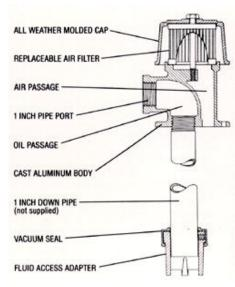
The **OIL**MISER™ FILLorDRAIN™ standardizes fluid handling procedures, at the very beginning of the contamination cycle. It closes the loop on airborne contamination from the drum to reservoir or from the reservoir to the drum.
