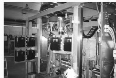
Illustration 1.13: Decentral motor controls integrated in packaging machine
