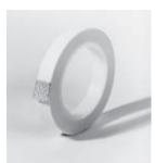
66' roll glass cloth installation tape with pressure sensitive thermosetting adhesive. 3/8" wide.  $310^{\circ}$ F ( $155^{\circ}$ C) rating. Strap at one foot intervals. Minimum application temperature  $40^{\circ}$ F ( $5^{\circ}$ C).
