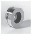
180' roll aluminum foil installation tape with pressure sensitive acrylic adhesive. 2-mil thickness with high tensile strength; 2-½" wide. 200°F (93°C) rating. Minimum application temperatures 40°F (5°C).
