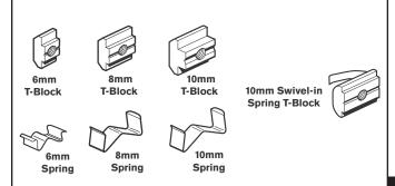
These T-slot Connectors can be used to fasten heavy components and accessories anywhere along the T-slot. The extra large contact surface with the inside of the profile provides a strong secure connection. All connectors can be easily repositioned in the T-slot. *T-blocks* slide into the end of the profile. The *Swivel-in T-block* with integrated spring can be installed anywhere along the T-slot.
