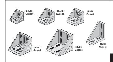
Die-cast *Gussets* connect profiles at right angles. Elongated holes allow gussets to be adjusted for position on the profile, while the alignment tabs assure proper location of the gusset in the profile T-slots. Alignment tabs can easily be removed with a flat-tip screwdriver when alignment with the T-slot is not desirable, such as when cross-connection of the profiles is required. All gussets will accept optional cover caps.
