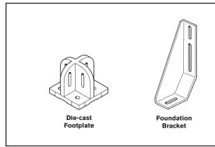
Heavy-duty die-cast aluminum *Foundation Brackets* allow you to secure structural profiles on machine bases, guarding and worktables to the shop floor using anchor bolts. Steel *Foundation Brackets* do not interfere with leveling feet and can be used to fasten structural profiles to floors, decks or shipping skids. Both are easy to attach to the profile with T-bolts.
