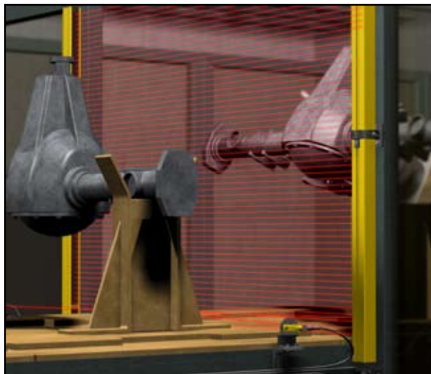
Figure 1-1. A typical EZ-SCREEN application: weld cell
